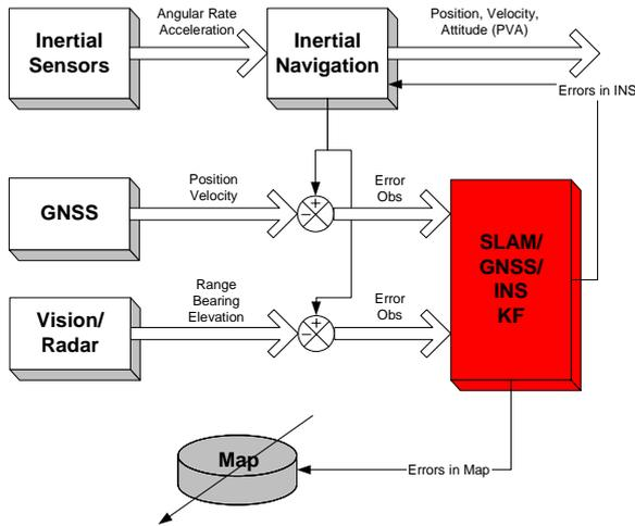
Fig. 2 The architecture of SLAM augmented GNSS/INS system
