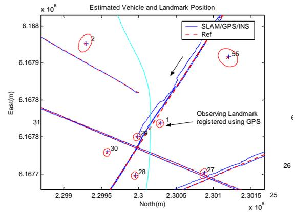
Figure 6. Enhanced view of INS correction by re-observing previously built map by GNSS.
