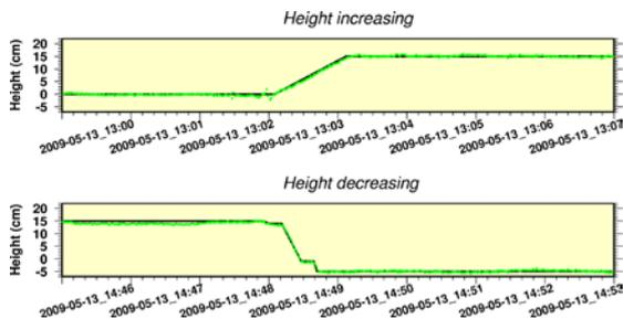
Fig. 6 Coordinate changes of station A17D in details during the height increasing and decreasing period, where the black lines represent the real track of the manual height changes and green dots are the real-time estimated coordinate changes compared to the true
