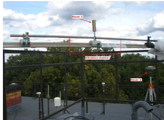
Fig. 2 The experiment field at GFZ, where Rover 1 (A17B) was set up on the horizontal linear table with scale panel to read the distances between the current and initial positions, and Rover 2 (A17D) was equipped with the device capable of adjusting the antenna height and recording the height changes
