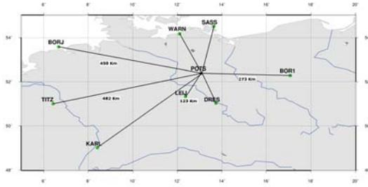
Fig. 3 Illustration of the real-time stations used in the experiment and the lengths of the baselines from the used reference stations to experiment kinematic stations in Potsdam, where POTB stands for A17B and A17D
