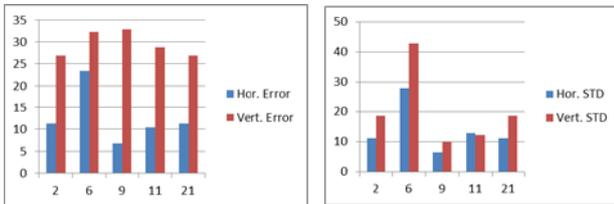
Figure 9e (i, ii) SET-Based AGNSS Mean Horizontal vs. Vertical Errors (left) and Standard Deviation (right)
