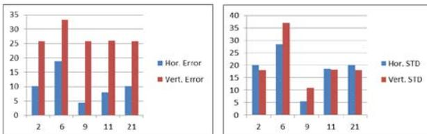
Figure 9f (i, ii) Stand-Alone GNSS Mean Horizontal vs. Vertical Errors (left) and Standard Deviation (right)
