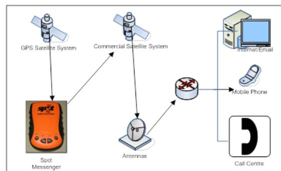
Figure 3: SPOT Satellite Messenger System
