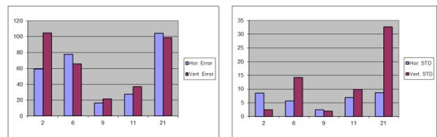
Figure 9c (i, ii) SPOT Messenger Mean Horizontal vs. Vertical Errors (left) and Standard Deviation (right)
