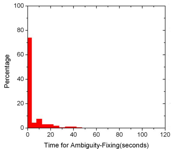
Figure 6 Observing time needed for ambiguity-fixing. 75% can be fixed within one epoch and on average two epoch data is needed.
