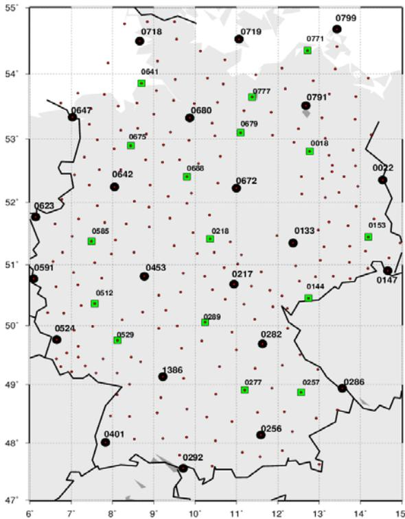
Figure 5 The German reference network and the SAPOS stations. Each small red dot indicates a real-time station of the SAPOS network. Large black dots indicate the selected regional reference stations and the large squares are for user stations.
