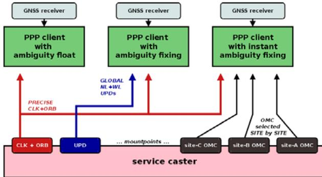
Figure 3 Data flow at the client side for standard PPP, PPP with ambiguity fixing and PPP with instantaneous ambiguity-fixing using regional augmentation information.
