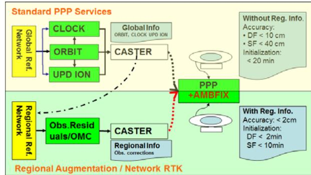
Figure 1 System structure of the global real-time precise positioning service based on Precise Point Positioning with the regional augmentation.
