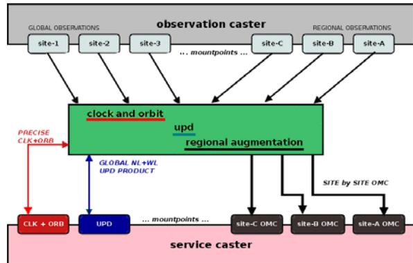
Figure 2 Data flow at the server side of the augmented global PPP service.
