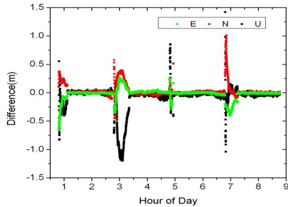
Figure 4 Impact of PPP ambiguity-fixing on position accuracy and convergence time. The estimator is restarted every two hours.
