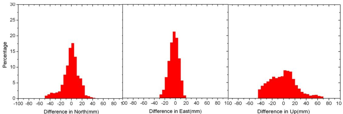
Figure 7 Distribution of position differences of the solutions with fixed ambiguities and the precise coordinates estimated in static mode.
