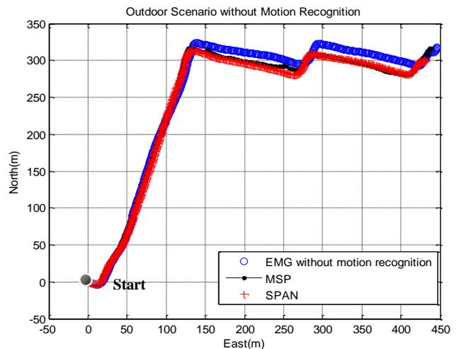
Figure 11. The trajectory of EMG PDR without motion recognition vs. commercial GPS receiver (with reference trajectory of SPAN) for outdoor scenario in a local coordinate.
