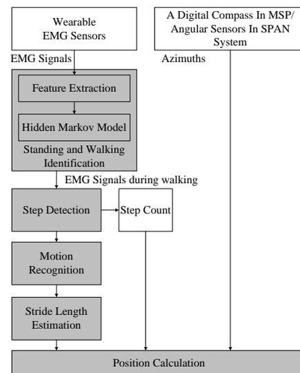
Figure 1. The diagram of the proposed EMG based pedestrian dead reckoning solution.
