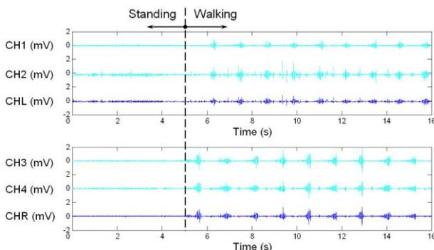
Figure 3. Typical raw EMG data collected when a tester is standing and then walking.
