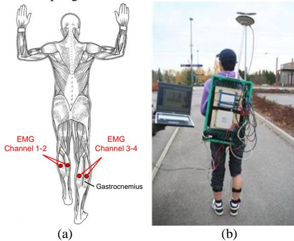
Figure 2. EMG sensors attached on the left and right leg (The background of (a) is obtained from <http://www.answers.com/topic/muscle>)
