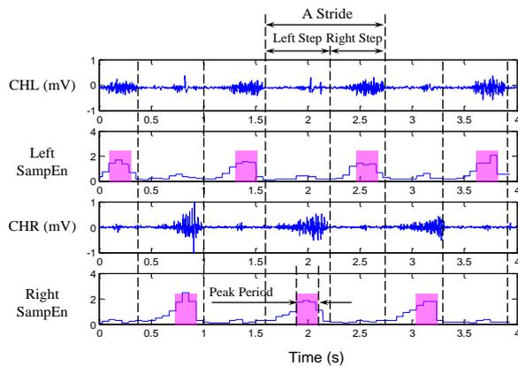
Figure 5. Illustration of step detection.
