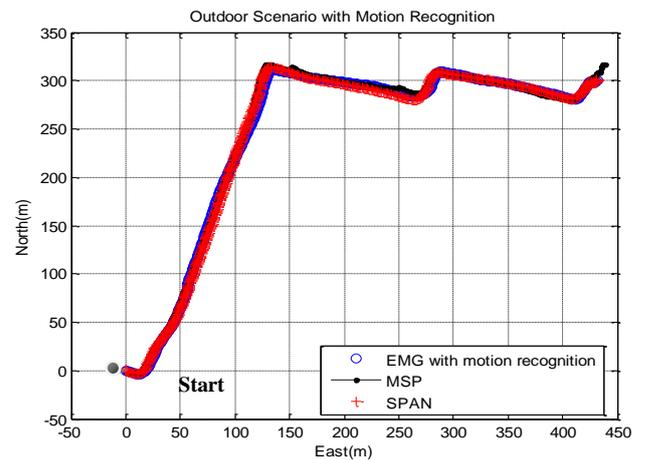
Figure 10. The trajectory of EMG PDR with motion recognition vs commercial GPS receiver (with reference trajectory of SPAN ) for outdoor scenario in a local coordinate.
