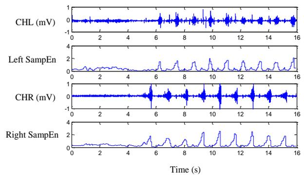
Figure 4. The sample entropy feature streams of the left and right legs respectively.
