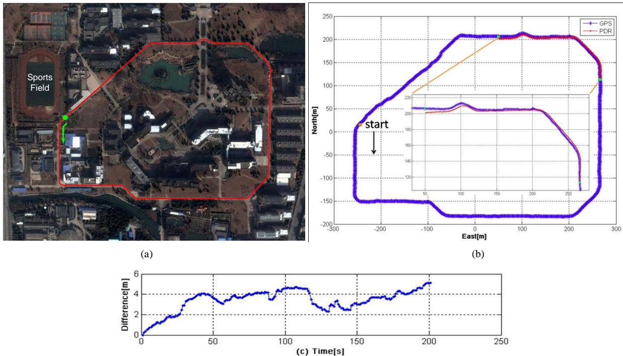
Figure 9. Positioning results of the simulated GPS outage gap: (a) the true route of the long-range test; (b) the PDR route of the simulated GPS outage gap against the GPS reference route; (c) Horizontal difference of the simulated GPS gap between the GPS and PDR solutions for about 200 seconds.
